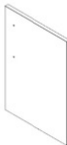
D2 PIZZA OVEN CABINET DOOR ASSEMBLY R - A4M03555 (x1) 28 7/16"x19 5/8"x15/16" (24x498x722.5)
