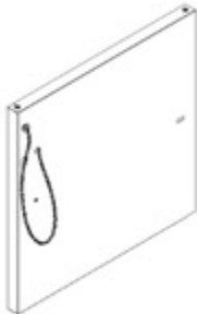
S6 GRILL CABINET SIDE PANEL ASSEMBLY M - A4M03586 (x1) 23 3/8"x22 7/8"x1 3/8" (35x581x593)
