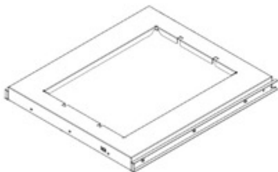
H3 TRASH CAN BRACKET ASSEMBLY - A4M03610 (x1) 18 1/16"x15 13/16"x (35x401.60x458)
