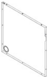
G3 SINK CABINET BACK PANEL ASSEMBLY - A4M03564 (x1) 34 5/16"x33 3/8"x1 3/16" (30x847.2x872)
