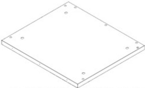
T7 FRIDGE CABINET TABLETOP - A4M03641 (x1) 27 3/8"x24 1/8"x1 1/4" (32x612x696)
