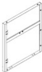
S14 PIZZA OVEN CABINET SIDE PANEL ASSEMBLY - A4M04536 (x1) 26 9/16"x23 3/8"x1 3/8" (35x594x675)
