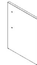
D8 CABINET DOOR ASSEMBLY R - A4M03590 (x1) 24 13/16"x19 1/16"x15/16" (24x484.15x630)
