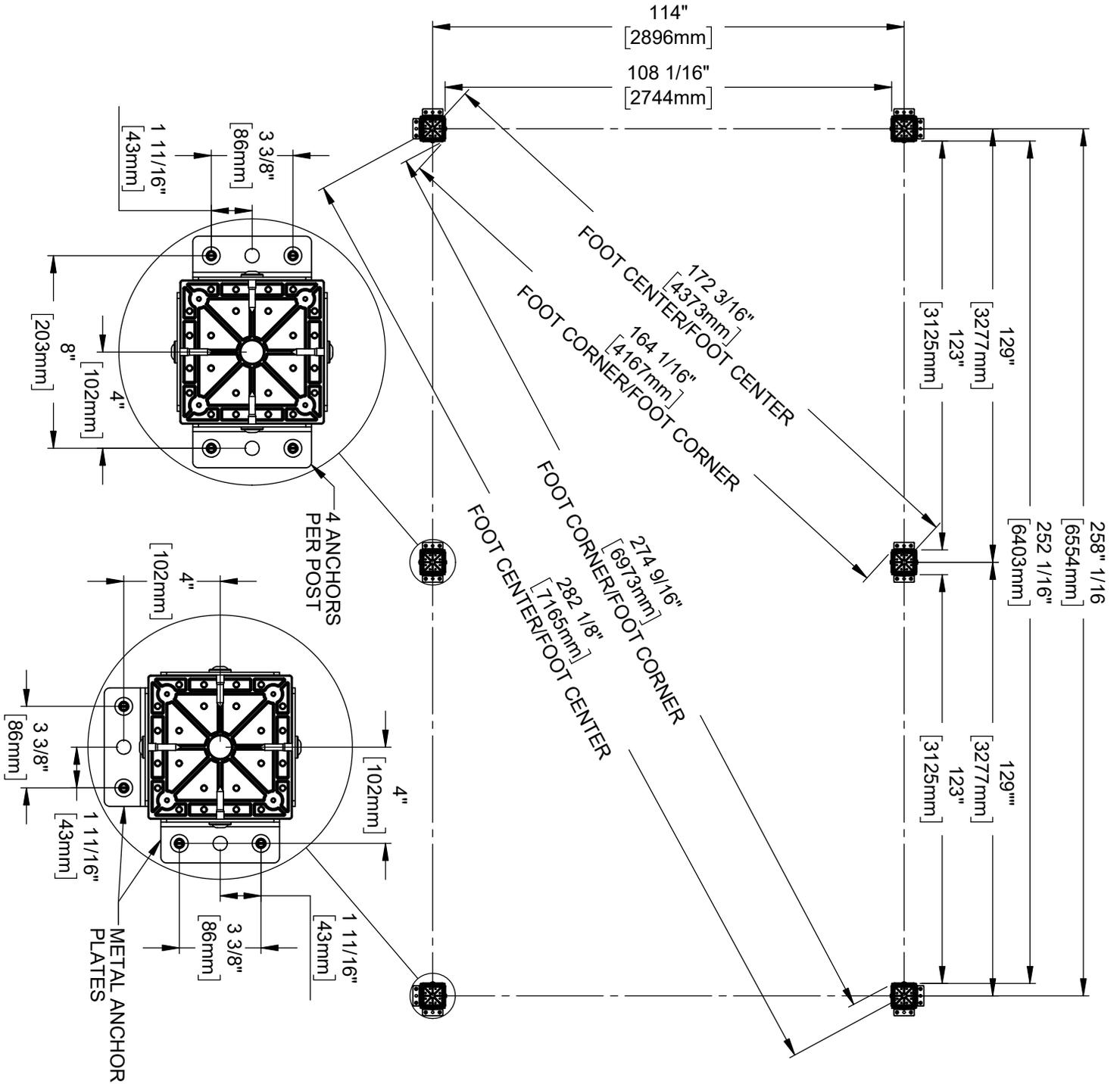
REMARQUE : LES DIMENSIONS SONT AUX PLAQUES D'ANCRAGE MONTÉES SUR LES POTEAUX SAUF SI INDIQUÉ DIFFÉREMENT
