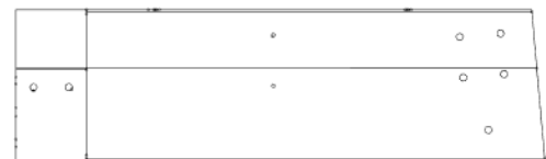
J12 JOIST ASSEMBLY - W2A04321 (x1) 1 7/16"x8 7/16"x29 1/2" (36x214x750)
