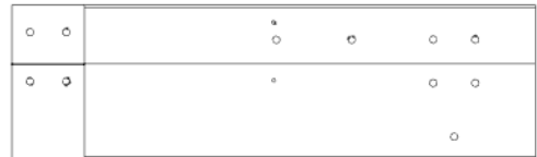
J06 BACK BEAM - W2A04318 (x1) 1 7/16"x8 7/16"x28 7/16" (36x214x722)
