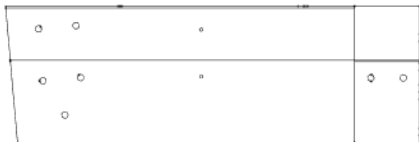
J11 JOIST ASSEMBLY - W2A04305 (x1) 1 7/16"x8 7/16"x25" (36x214x635)
