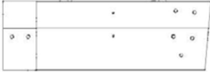
J14 JOIST ASSEMBLY - W2A04322 (x1) 1 7/16"x8 7/16"x25" (36x214x635)
