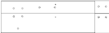
J01 JOIST END ASSEMBLY - W2A04471 (x1) 1 7/16"x8 7/16"x28 7/16" (36x214x722)
