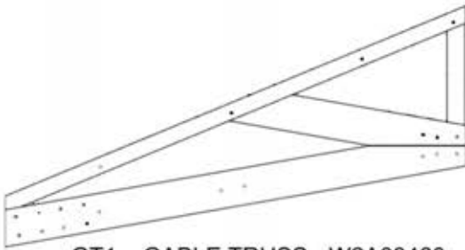
GT1 GABLE TRUSS - W2A03460 (x4) 1 3/8"x34"x64 5/8" (36x864x1640)
