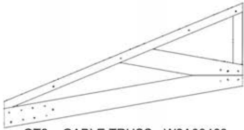
GT2 GABLE TRUSS - W2A03463 (x2) 1 3/8"x34"x64 5/8" (36x864x1640)
