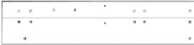
J01 JOIST END ASSEMBLY - W2A04462 (x2) 15/16"x8 7/16"x37 1/8" (24x214x943)
