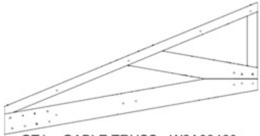
GT1 GABLE TRUSS - W2A03460 (x2) 1 3/8"x34"x64 5/8" (36x864x845)
