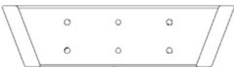
H11 ROOF JOIST - W4L16801 (x1) 15/16"x3 3/8"x12 15/16" (24x86x328)
