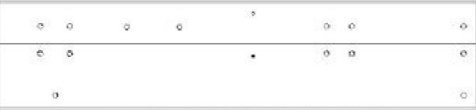
J06 JOIST END ASSEMBLY - W2A04464 (x2) 15/16"x8 7/16"x37 1/8" (24x214x943)
