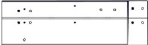
J01 JOIST ASSEMBLY - W2A03549 (x1) 1 7/16"x8 7/16"x28 7/16" (36x214x722)
