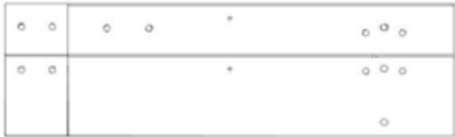
J06 JOIST ASSEMBLY - W2A03552 (x1) 1 7/16"x8 7/16"x28 7/16" (36x214x722)
