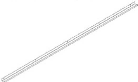
G03 GUTTER - A4M02571 (x2) 1 9/16"x1 15/16"x92 7/8" (40x50x2359)
