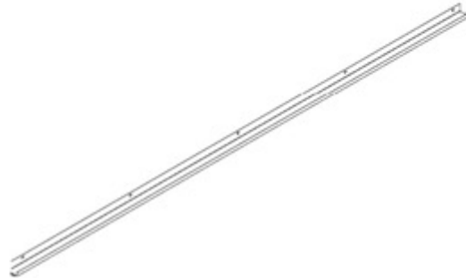
G02 GUTTER - A4M02570 (x2) 1 9/16"x1 15/16"x92 7/8" (40x50x2359)
