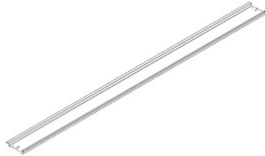
L01 LOUVER ASSEMBLY - A4M01995 (x28) 1 11/16"x7 3/4"x114 5/16" (42x196x2904)
