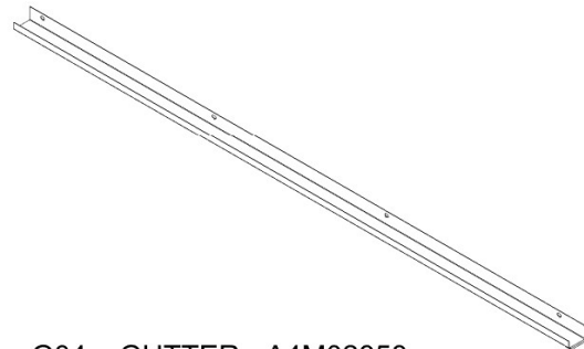
G04 GUTTER - A4M02858 (x2) 1 9/16"x1 15/16"x65 15/16" (40x50x1675)
