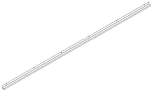
G01 GUTTER - A4M01993 (x2) 1 9/16"x1 15/16"x108 7/8" (40x50x2765)
