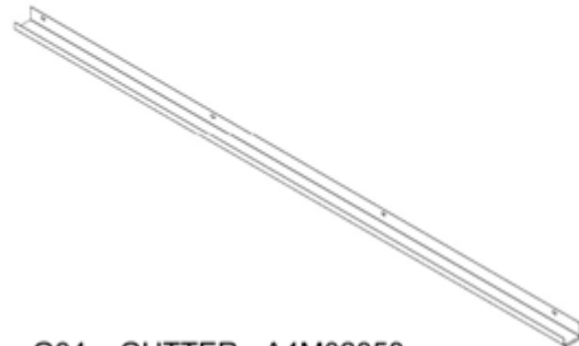
G04 GUTTER - A4M02858 (x2) 1 9/16"x1 15/16"x65 15/16" (40x50x1675)
