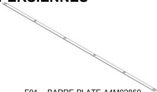
F01 BARRE PLATE-A4M02859 (x4) 1/16"x1"x65 7/8" (2x25x1673)
