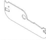
L03 LOUVER SIDE PLATE - A4M04138 (x38) 1/16"x2 3/16"x6 9/16" (2x55x167)
