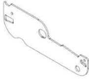
L02 LOUVER DRIVE SIDE PLATE - A4M04139 (x1) 1/16"x2 3/16"x6 9/16" (2x55x167)
