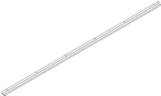
G01 GUTTER - A4M01993 (x2) 1 9/16"x1 15/16"x108 7/8" (40x50x2765)
