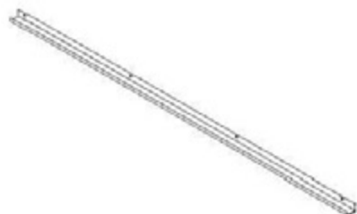
G04 GUTTER - A4M01999 (x1) 1 9/16"x1 15/16"x79 7/16" (40x50x2017)
