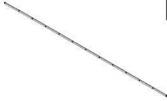
F02 LOUVER TIE STRAP - A4M02130 (x1) 1/8"x5/8"x81 7/16" (3x16x2068)
