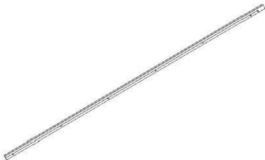
G02 GUTTER - A4M03481 (x1) 1 9/16"x1 15/16"x1117 5/16" (40x50x2838)
