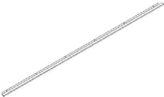
G01 GUTTER - A4M03478 (x1) 1 9/16"x1 15/16"x1117 5/16" (40x50x2838)
