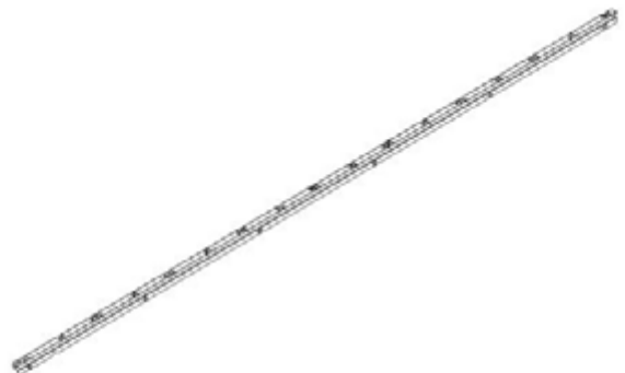
M02 LOUVER MOUNT - A4M02594 (x2) 1"x1 15/16"x110 3/4" (25x49x2813)
