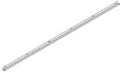
G06 GUTTER - A4M03481 (x2) 1 9/16"x1 15/16"x111 3/4" (40x50x2839)
