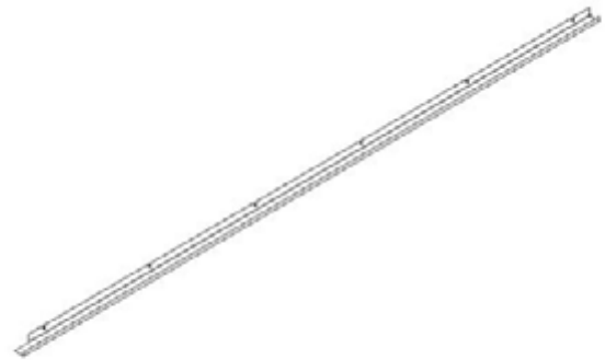
G02 GUTTER - A4M02583 (x1) 1 9/16"x1 15/16"x1111" (40x50x2820)
