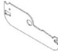
L03 LOUVER SIDE PLATE - A4M04138 (x64) 1/16"x2 3/16"x6 9/16" (2x55x167)
