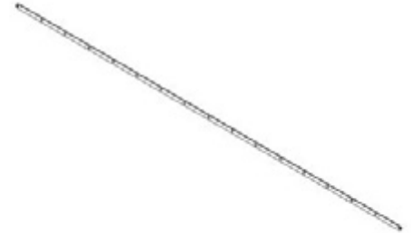
F02 LOUVER TIE STRAP - A4M04059 (x4) 1/8"x13/16"x108 3/8" (3x20x2752)
