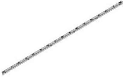
M02 LOUVER MOUNT - A4M02594 (x1) 1"x1 15/16"x110 3/4" (25x49x2813)
