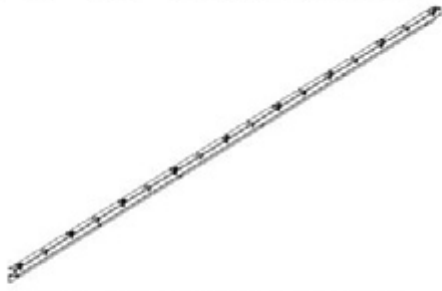
M02 LOUVER MOUNT - A4M02594 (x1) 1"x1 15/16"x110 3/4" (25x49x2813)
