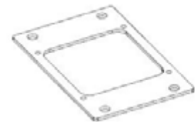
SHIM - A4M04024 (x6) 1/8"x4 3/8"x6 3/4" (3x110x172)
