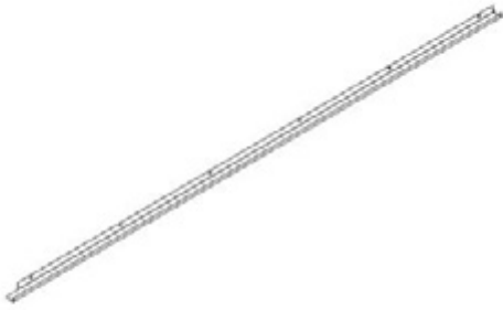
G02 GUTTER - A4M02583 (x1) 1 9/16"x1 15/16"x111" (40x50x2820)
