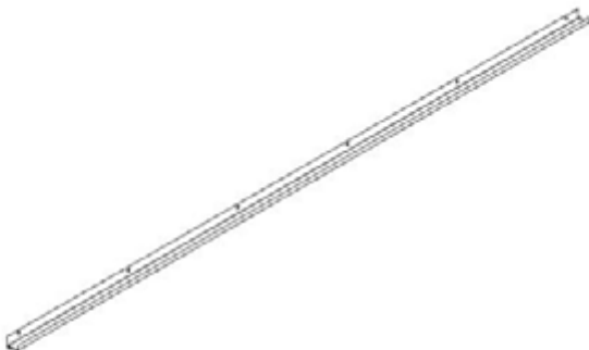
G06 GUTTER - A4M03481 (x2) 1 9/16"x1 15/16"x1111 3/4" (40x50x2839)
