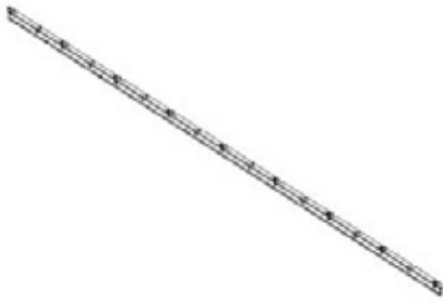
M04 LOUVER MOUNT - A4M02596 (x2) 1"x1 15/16"x110 3/4" (25x49x2813)
