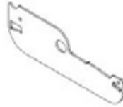
L03 LOUVER SIDE PLATE - A4M04138 (x66) 1/16"x2 3/16"x6 9/16" (2x55x167)
