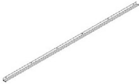
G02 GUTTER - A4M02583 (x1) 19/16"x1 15/16"x111" (40x50x2820)
