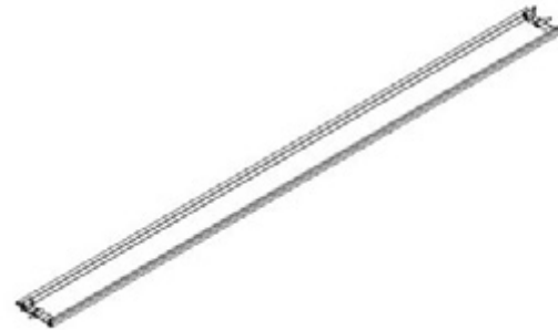
L01 LOUVER - A4M04137 (x34) 1 11/16"x7 5/8"x114 5/16" (42x194x2904)
