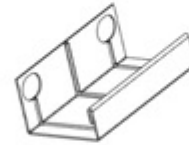
G05 GUTTER SPLICE - A4M02004 (x2) 1 7/16"x2 1/16"x3 15/16" (36x52.5x100)
