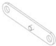
F03 LINKAGE STRAP - A4M02229 (x1) 1/8"x11/16"x3 13/16" (13x17x97)
