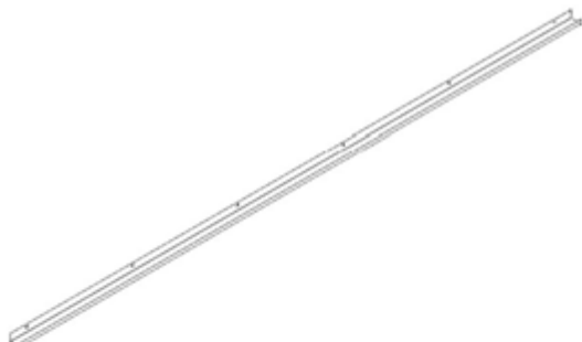
G01 GUTTER - A4M01993 (x2) 1 9/16"x1 15/16"x108 7/8" (40x50x2765)
