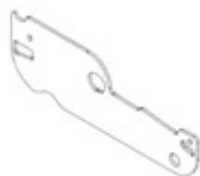
L02 LOUVER DRIVE SIDE PLATE - A4M04139 (x1) 1/16"x2 3/16"x6 9/16" (2x55x167)
