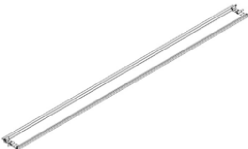
L01 LOUVER - A4M04137 (x20) 1 11/16"x7 3/4"x114 5/16" (42x196x2904)
