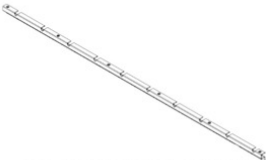
M02 LOUVER MOUNT - A4M02865 (x1) 1"x1 15/16"x65 7/8" (25x49x1673)
