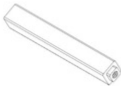
L02 LOUVER DRIVE SIDE PLATE - A4M04139 (x1) 1/16"x2 3/16"x6 9/16" (2x55x167)
