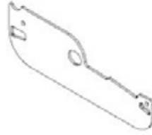
L03 LOUVER SIDE PLATE - A4M04138 (x33) 1/16"x2 3/16"x6 9/16" (2x55x167)
