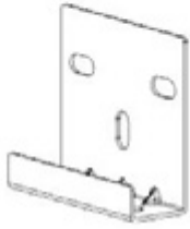
K03 WALL BRACKET - A4M03482 (x1) 2 11/16"x5 3/16"x6" (69x131x152)
