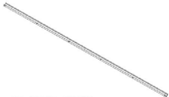
G03 GUTTER - A4M04120 (x1) 1 9/16"x1 15/16"x111 11/16" (40x50x2837)
