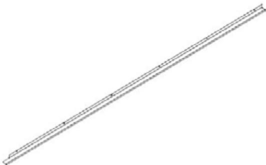
G02 GUTTER - A4M03481 (x1) 1 9/16"x1 15/16"x111 13/16" (40x50x2839)
