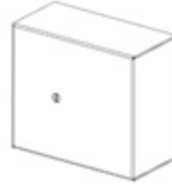
L03 LOUVER SIDE PLATE - A4M04138 (x39) 1/16"x2 3/16"x6 9/16" (2x55x167)
