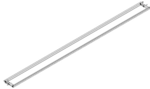
L01 LOUVER - A4M04137 (x20) 1 11/16"x7 3/4"x114 5/16" (42x196x2904)
