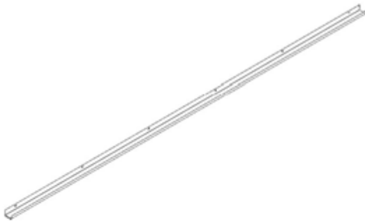
G01 GUTTER - A4M01993 (x2) 1 9/16"x1 15/16"x108 7/8" (40x50x2765)
