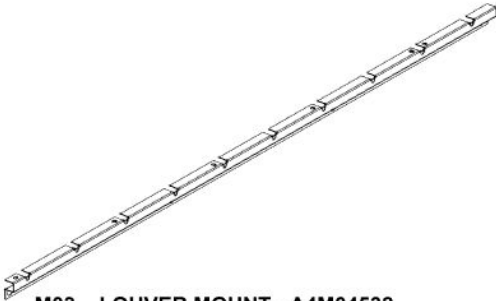
M03 LOUVER MOUNT - A4M04532 (x1) 1"x1 15/16"x65 13/16" (25x48.5x1672)
