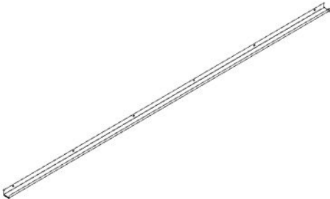
G01 GUTTER - A4M01993 (x1) 1 9/16"x1 15/16"x108 7/8" (40x50x2765)
