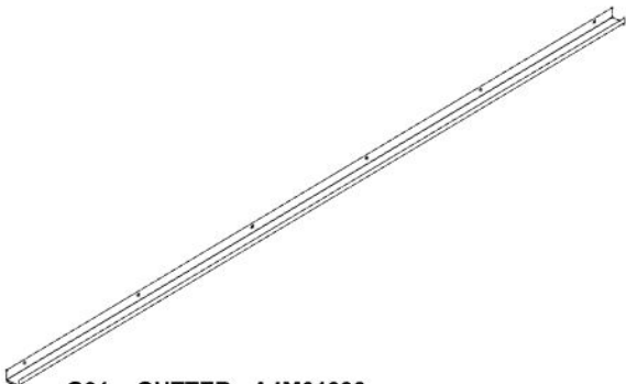
G01 GUTTER - A4M01993 (x2) 1 9/16"x1 15/16"x108 7/8" (40x50x2765)
