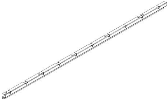
M03 LOUVER MOUNT - A4M04532 (x2) 1"x1 15/16"x65 13/16" (25x48.5x1672)
