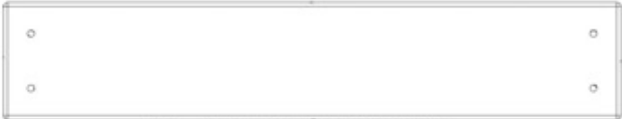
M03 SPIGOT BOARD - W4L20219 (x1) 5/8"x3 3/8"x17 11/16" (16x86x450)
