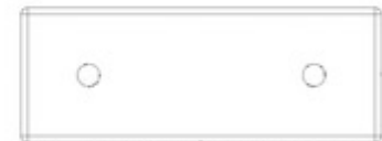
N02 SPACER BOARD - W4L20183 (x1) 5/8"x2 3/8"x6 5/16" (16x60x160)
