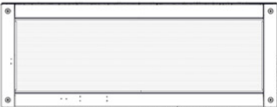
WA01 WINDOW ASSEMBLY - W2A04344 (x1) 1 7/8"x17 1/2"x47 3/16" (48x444x1198)
