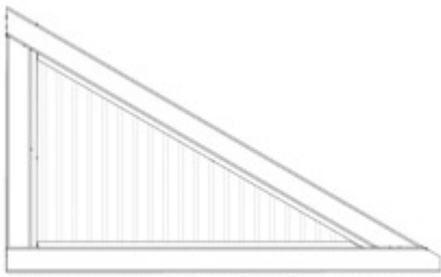
WA02 WINDOW ASSEMBLY - W2A04190 (x1) 1 7/16"x15 11/16"x24 3/4" (36x398x629)
