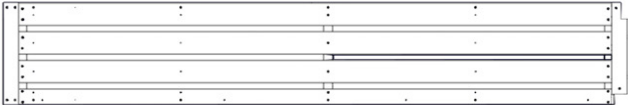
TB01 TABLE ASSEMBLY - W2A04187 (x1) 2 1/16"x14 7/8"x89 1/2" (52x378x2274)
