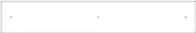
Y01 COVER BOARD - W4L19679 (x2) 5/8"x4"x24 3/16" (16x102x614)
