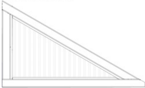
WA02 WINDOW ASSEMBLY - W2A04190 (x2) 1 7/16"x15 11/16"x24 3/4" (36x398x629)
