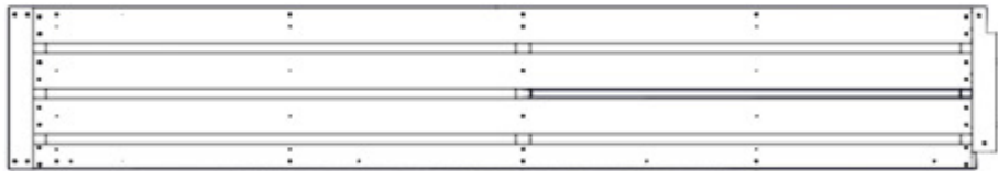
TB01 TABLE ASSEMBLY - W2A04187 (x1) 2 1/16"x14 7/8"x89 1/2" (52x378x2274)
