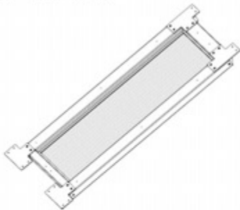
WINDOW ASSEMBLY WITH CLEATS FROM STEP 120
