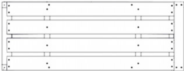
TB08 TABLE ASSEMBLY - W2A04389 (x1) 2 1/16"x16 1/16"x42 5/8" (52x408x1083)
