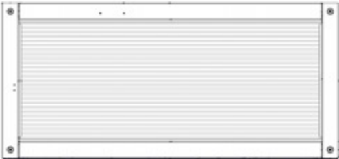
WA06 WINDOW ASSEMBLY - W2A04205 (x1) 1 7/8"x21 13/16"x47 3/16" (48x554x1094)
