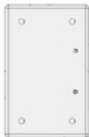
K04 LATCH BLOCK - W4L19789 (x2) 5/8"x3"x4 3/4" (16x76x120)
