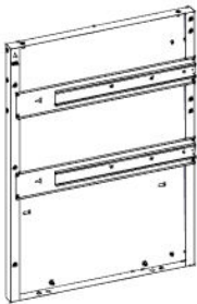
S31 CABINET SIDE PANEL ASSEMBLY - A4M04838 (x1) 33 3/8"x23 3/8"x1 15/16" (49.00x594x848.20)
