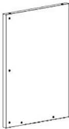
S29 CABINET SIDE PANEL ASSEMBLY - A4M04833 (x1) 33 3/8"x23 3/8"x1 3/8" (35.00x594x848.20)
