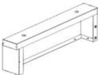
T5 CABINET COUNTERTOP PANEL ASSEMBLY L - A4M04537 (x1) 24 1/8"x4 5/16"x6 3/4" (109x172.2x612)
