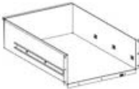
D4 CABINET DRAWER BODY ASSEMBLY - A4M03571 (x2) 22 1/4"x16 1/16"x6 7/16" (164.2x408.4x565.4)
