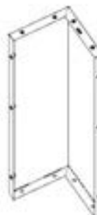
S34 CABINET CORNER PANEL ASSEMBLY - A4M04850 (x1) 33 3/8"x8 11/16"x8 11/16" (220x220x848)
