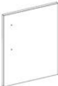
D8 CABINET DOOR ASSEMBLY R - A4M03590 (x1) 24 13/16"x19 1/16"x15/16" (24x484.15x630)
