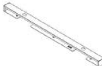
A14 COUNTERTOP BRACKET ASSEMBLY - A4M04846 (x1) 24 3/16"x1 3/8"x1 1/4" (31.00x35.00x614.00)
