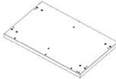
F3 CABINET FLOOR PANEL ASSEMBLY - A4M03560 (x1) 37 3/16"x23 3/8"x2 5/8" (66x594x944)
