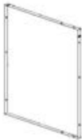
G14 CABINET BACK PANEL ASSEMBLY - A4M04716 (x1) 27 5/16"x33 3/8"x1 3/16" (30x847.2x693)
