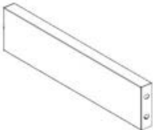
H16 CABINET HORIZONTAL BEAM ASSEMBLY - A4M04719 (x1) 14 5/8"x3 3/8"x1" (25x85x372)
