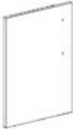
D1 CABINET DOOR PANEL ASSEMBLY L - A4M03546 (x1) 28 7/16"x19 5/8"x15/16" (24x498x722.5)
