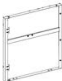
S14 CABINET SIDE PANEL ASSEMBLY - A4M04536 (x1) 26 9/16"x23 3/8"x1 3/8" (35x594x675)
