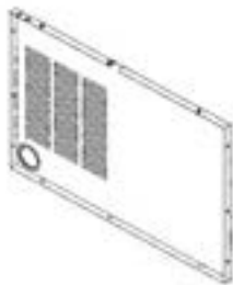
G1 CABINET BACK PANEL ASSEMBLY - A4M03542 (x1) 38 3/4"x26 1/2"x1 3/16" (30x673.5x984)
