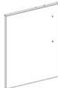
D7 CABINET DOOR ASSEMBLY L - A4M03587 (x1) 24 13/16"x19 1/16"x15/16" (24x484.15x630)
