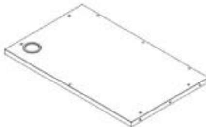
T13 TABLETOP ASSEMBLY - A4M04668 (x1) 1 1/4"x23 3/8"x38 3/16" (32x594x970)
