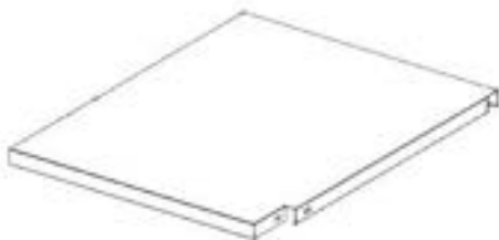
L2 CABINET SHELF ASSEMBLY - A4M03589 (x1) 23 1/4"x18 3/8"x1" (25.00x467.00x591.00)
