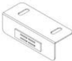
A2 MAGNET BRACKET - A4M03026 (x7) 1"x1 1/4"x3 1/8" (25x31x80)
