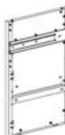
S36 CABINET SIDE PANEL ASSEMBLY L - A4M04852 (x1) 33 3/8"x23 3/8"x1 3/8" (35.00x594.00x848.20)
