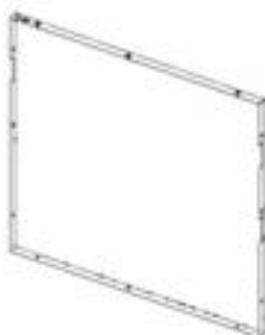
G15 CABINET BACK PANEL ASSEMBLY - A4M04707 (x1) 34 5/16"x33 3/8"x1 3/16" (30x847.2x1049)
