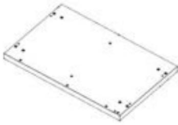
F3 CABINET FLOOR PANEL ASSEMBLY - A4M03560 (x1) 37 3/16"x23 3/8"x2 5/8" (66x594x944)
