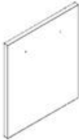
D9 CABINET TRASH CAN PANEL ASSEMBLY - A4M03608 (x1) 22 1/4"x17 3/4"x15/16" (24.00x451.00x565.00)
