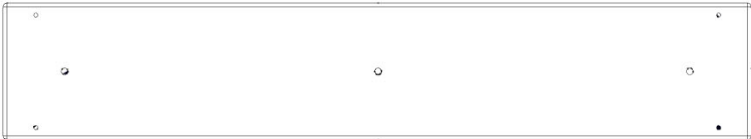
AD01 ELECTRICAL ENCLOSURE BOARD - W4L20755 (x1) 15/16"x4"x22 1/16" (24x102x560)
