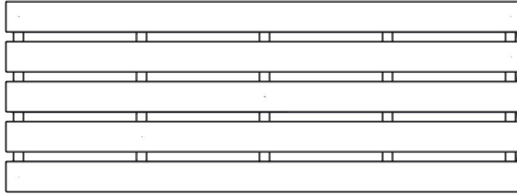
FP01 FLOOR PANEL ASSEMBLY - W2A04796 (x1) 1 15/16"x20 7/8"x55 7/8" (50x530x1420)
