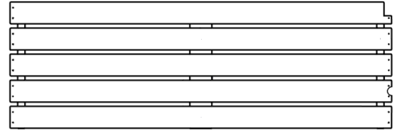
BA02 LEFT BENCH ASSEMBLY - W2A04789 (x1) 19 1/8"x57 5/16" (50x486x1456)
