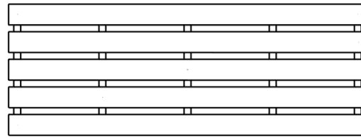
FP01 FLOOR PANEL ASSEMBLY - W2A04796 (x1) 1 15/16"x20 7/8"x55 7/8" (50x530x1420)
