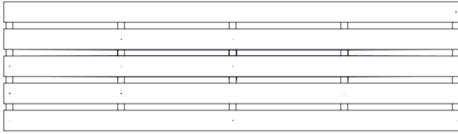
FP01 FLOOR PANEL ASSEMBLY - W2A04829 (x1) 1 15/16"x20 7/8"x73 7/8" (50x530x1876)
