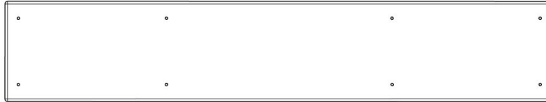
OV01 HEATER GUARD SPACER - W4L21887 (x2) 1 3/16"x4 7/16"x23 15/16" (30x112x608)
