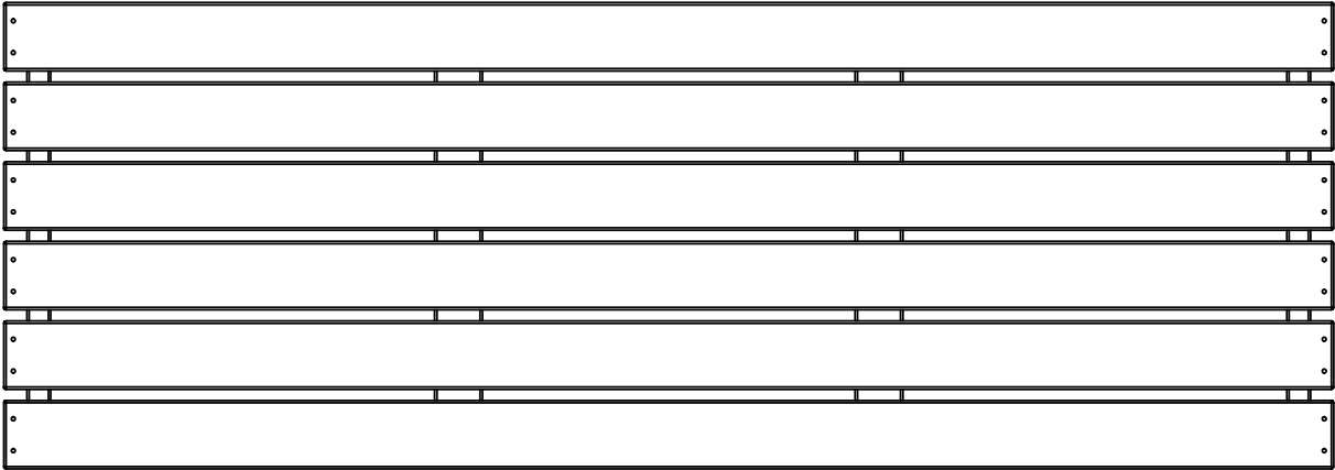
BA02 BENCH ASSEMBLY-W2A04822 (x1) 1 15/16"x23 1/16"x65 3/4" (50x586x1670)
