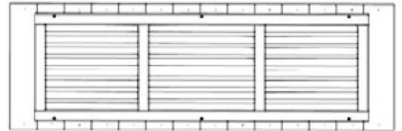
P04 SEAT SUPPORT PANEL RIGHT - W2A04898 (x1) 2 11/16"x15 3/8"x46 3/4" (69x390x1187)
