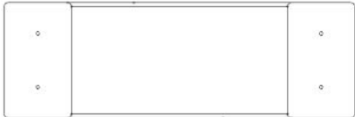
W02 FOOT BRACE - W4L22399 (x3) 1 15/16"x3 3/8"x10 1/4" (50x86x261)
