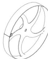
W01 WHEEL ASSEMBLY - A4M02146 (x1) 2 3/8"x7" (59.7x178)
