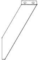
C03 BRACE - A4M05262 (x3) 1 7/16"x5 15/16"x27 1/8" (36x151x688)
