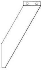
C05 BRACE WITH TAG - A4M05860 (x1) 1 7/16"x5 15/16"x27 1/8" (36x151x688)
