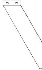
C04 BRACE - A4M05263 (x1) 1 7/16"x5 15/16"x27 1/8" (36x151x688)
