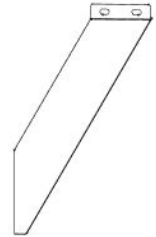
C05 BRACE WITH TAG - A4M05860 (x1) 1 7/16"x5 15/16"x27 1/8" (36x151x688)
