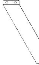
C04 BRACE - A4M05263 (x4) 1 7/16"x5 15/16"x27 1/8" (36x151x688)
