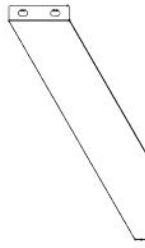
C04 BRACE - A4M05263 (x3) 1 7/16"x5 15/16"x27 1/8" (36x151x688)
