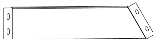
B09 GABLE SUPPORT - A4M04319 (x2) 1 1/2"x5 15/16"x24 5/8" (38x152x625)
