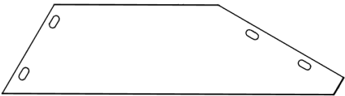
C05 ANGLE BRACE - A4M04320 (x2) 1 7/16"x5 5/16"x20 1/16" (36x135x509)
