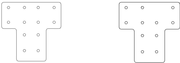
A4M04104 POST SUPPORT BRACKET (x2)
