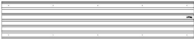
3528 STEEL SHEETING - A4M03528 (x8) 87"x18 7/8"x1/4" (7x480x2210)
