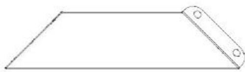
C02 CORBEL ASSEMBLY - A4M03526 (x1) 21 13/16"x5 1/4"x2 3/4" (70x134x553.5)
