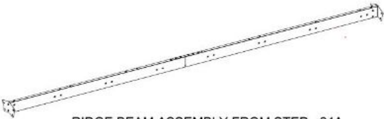
RIDGE BEAM ASSEMBLY FROM STEP - 24A
