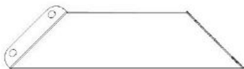
CO1 ASSEMBLAGE DE CORBEAU - A4M03525 (x1) 2113/16"x5 1/4"x2 3/4" (70x134x553.5)
