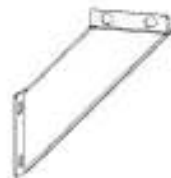
C02 CORBEL ASSEMBLY - A4M05702 (x4) 12 1/4"x3 3/4"x1 15/16" (50x96x309)
