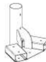
FB01 FRAME BRACKET ASSEMBLY - A4M06615 (x1) 12 3/4"x8 7/8"x13 7/8" (352x227x324)
