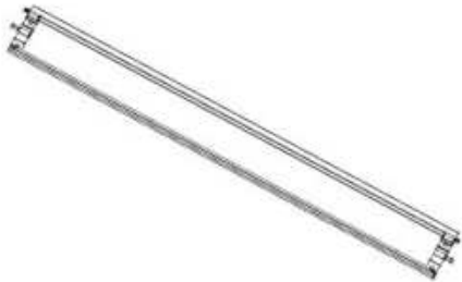
L01 LOUVER - A4M06326 (x24) 1 11/16"x7 3/4"x67 15/16" (42x196.2x1726.5)
