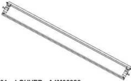
L01 LOUVER - A4M06326 (x1) 1 11/16"x7 3/4"x67 15/16" (42x196.2x1726.5)
