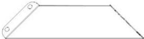
C01 CORBEL ASSEMBLY - A4M03525 (x1) 21 13/16"x5 1/4"x2 3/4" (70x134x553.5)
