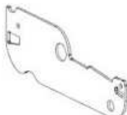
L02 LOUVER DRIVE SIDE PLATE - A4M04139 (x4) 1/16"x2 3/16"x6 9/16" (2x55x167)
