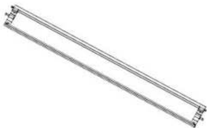
L01 LOUVER - A4M06326 (x52) 1 11/16"x7 3/4"x67 15/16" (42x196.2x1726.5)
