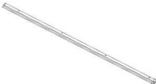
G05 GUTTER - A4M06328 (x2) 1 11/16"x3 1/8"x87 5/16" (43x80x2218)
