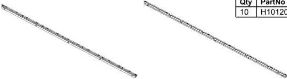
M02 LOUVER MOUNT - A4M05831 (x1) 1"x1 15/16"x88 1/4" (25x49x2241)
