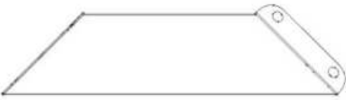
C02 CORBEL ASSEMBLY - A4M03526 (x1) 21 13/16"x5 1/4"x2 3/4" (70x134x553.5)
