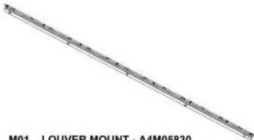
M01 LOUVER MOUNT - A4M05830 (x2) 1"x1 15/16"x88 1/4" (25x49x2241)
