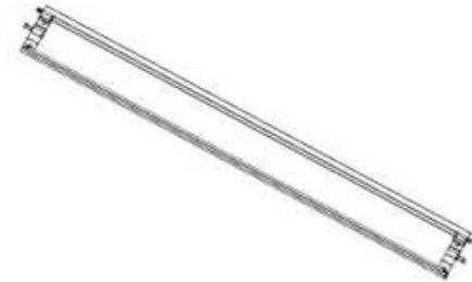
L01 LOUVER - A4M06326 (x1) 1 11/16"x7 3/4"x67 15/16" (42x196.2x1726.5)
