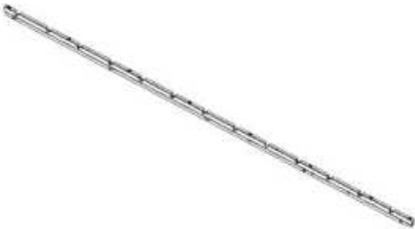
M01 LOUVER MOUNT - A4M05830 (x1) 1"x1 15/16"x88 1/4" (25x49x2241)
