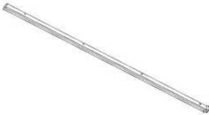
G05 GUTTER - A4M06328 (x1) 1 11/16"x3 1/8"x87 5/16" (43x80x2218)
