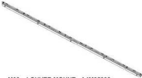
M03 LOUVER MOUNT - A4M05832 (x2) 1"x1 15/16"x88 1/4" (25x49x2241)
