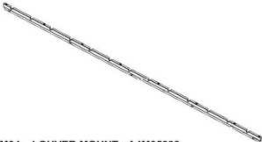
M04 LOUVER MOUNT - A4M05833 (x2) 1"x1 15/16"x88 1/4" (25x49x2241)
