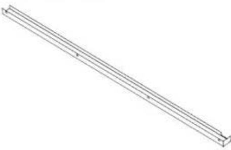
G08 GUTTER - A4M06480 (x1) 1 3/4"x2 11/16"x76 1/2" (50.00x69x1943)
