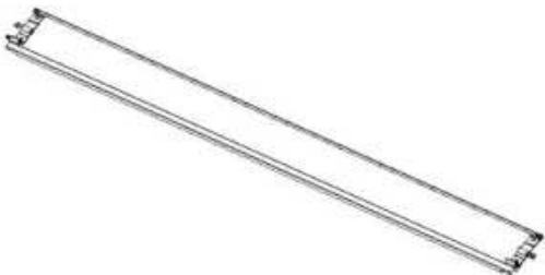
L06 LOUVER - A4M06474 (x52) 1 11/16"x7 3/4"x80" (42x196.2x2031.5)
