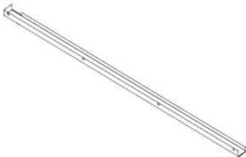
G07 GUTTER - A4M06479 (x2) 1 15/16"x2 11/16"x76 1/2" (50x69x1943)
