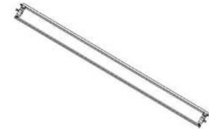
L06 LOUVER - A4M06474 (x1) 1 11/16"x7 3/4"x80" (42x196.2x2031.5)
