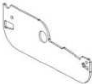
L03 LOUVER SIDE PLATE - A4M04138 (x1) 1/16"x2 3/16"x6 9/16" (2x55x167)
