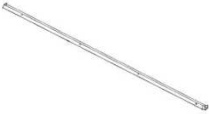
G06 GUTTER - A4M06329 (x1) 1 11/16"x3 1/8"x87 5/16" (43x80x2218)
