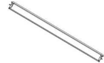
L06 LOUVER - A4M06474 (x1) 1 11/16"x7 3/4"x80" (42x196.2x2031.5)
