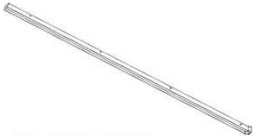
G05 GUTTER - A4M06328 (x2) 1 11/16"x3 1/8"x87 5/16" (43x80x2218)
