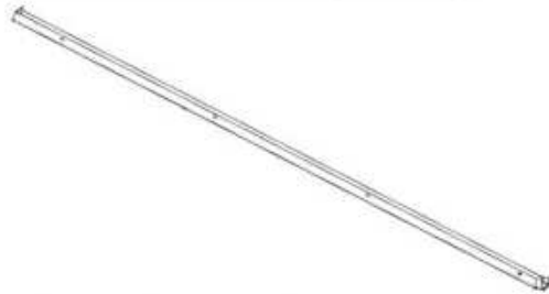
G06 GUTTER - A4M06329 (x2) 1 11/16"x3 1/8"x87 5/16" (43x80x2218)
