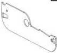
L03 LOUVER SIDE PLATE - A4M04138 (x48) 1/16"x2 3/16"x6 9/16" (2x55x167)
