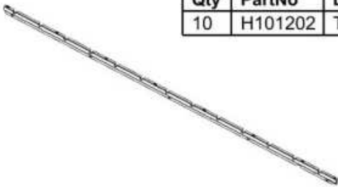
M04 LOUVER MOUNT - A4M05833 (x1) 1"x1 15/16"x88 1/4" (25x49x2241)
