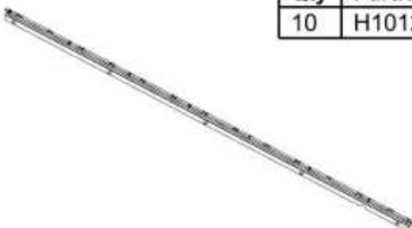
M03 LOUVER MOUNT - A4M05832 (x1) 1"x1 15/16"x88 1/4" (25x49x2241)
