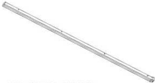
G05 GUTTER - A4M06328 (x2) 1 11/16"x3 1/8"x87 5/16" (43x80x2218)
