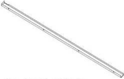
G09 GUTTER - A4M06489 (x1) 1 15/16"x2 11/16"x88 1/2" (50x69x2248)
