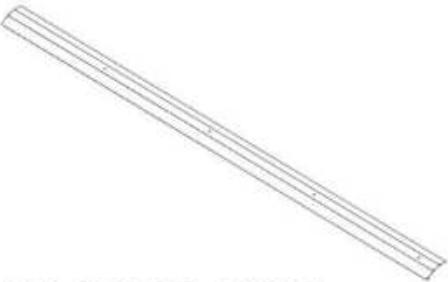
6493 RIDGE CAP - A4M06493 (x2) 3/4"x5 3/8"x94 7/16" (19x137x2398)
