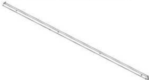
G06 GUTTER - A4M06329 (x2) 1 11/16"x3 1/8"x87 5/16" (43x80x2218)
