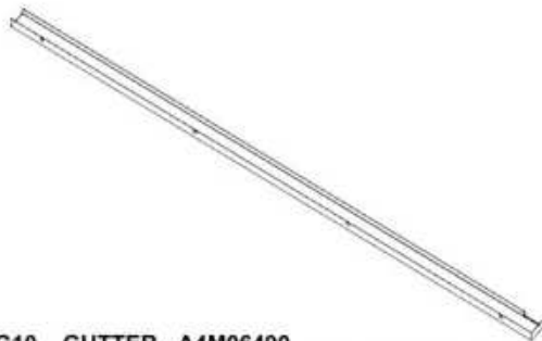
G10 GUTTER - A4M06490 (x2) 1 3/4"x2 11/16"x88 1/2" (50.00x69x2248)
