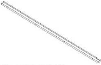
G10 GUTTER - A4M06490 (x1) 1 3/4"x2 11/16"x88 1/2" (50.00x69x2248)
