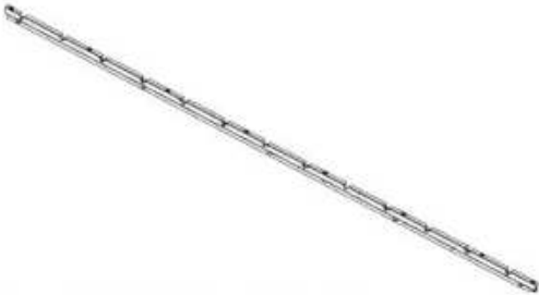
M02 LOUVER MOUNT - A4M05831 (x2) 1"x1 15/16"x88 1/4" (25x49x2241)
