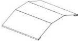
5826 RIDGE CAP SPLICE - A4M05826 (x1) 7/8"x3 15/16"x5 1/2" (21.5x139x100)
