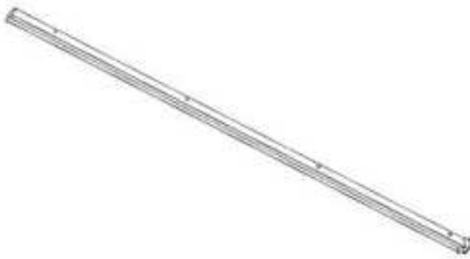
G05 GUTTER - A4M06328 (x1) 1 11/16"x3 1/8"x87 5/16" (43x80x2218)
