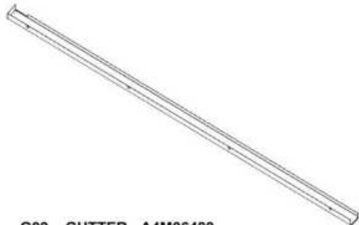
G09 GUTTER - A4M06489 (x2) 1 15/16"x2 11/16"x88 1/2" (50x69x2248)
