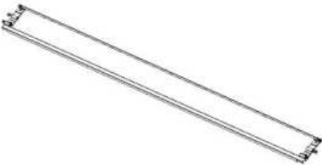
L05 LOUVER - A4M06484 (x24) 1 11/16"x7 3/4"x91 15/16" (42x196.2x2336.5)
