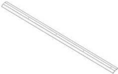
6493 RIDGE CAP - A4M06493 (x1) 3/4"x5 3/8"x94 7/16" (19x137x2398)
