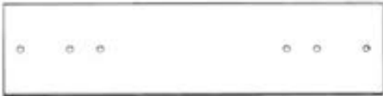
W14 ROCK WALL BOARD - A5C00009 (x2) 29 5/16"x5 1/2"x7/8" (23x140x744)
