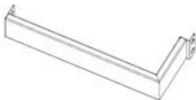
FR04 FLOOR RAIL ASSEMBLY - A4M05944 (x2) 18"x7 1/8"x3 1/8" (80x182x459)
