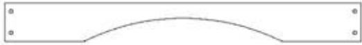
L5 | GUÍA DE PARED DE LA CASA CLUB - W4L14567 (x1) 5/8" x 4 3/8" x 40 3/8" (16 x 112 x 1024)
