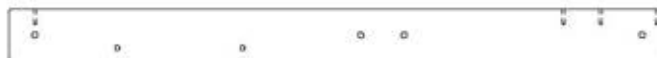
E8 | PATA DE LA CASA CLUB - W4L14537 (x1) | 1 3/8" x 3 3/8" x 43 1/8" (36 x 86 x 1094)
