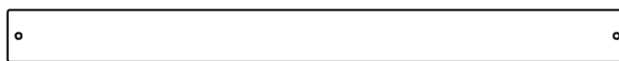
M13 | LISSE MURALE - W103973 (x1) | 5/8 po x 3 3/8 po x 40 3/8 po (16 x 86 x 1024)
