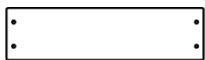
M4 | LAMELLE MURALE - W103995 (x5) | 5/8 po x 3 3/8 po x 12 7/8 po (16 x 86 x 326)
