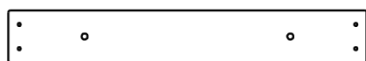
M26 | PLANCHE DE FIXATION - W4L16334 (x1) | 1 po x 3 3/8 po x 23 1/4 po (24 x 86 x 592)
