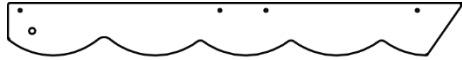
H3 | SUPPORT DE TOIT - W104017 (x2) | 1 po x 3 3/8 po x 29 5/8 po (24 x 86 x 752)
