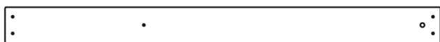
M24 | LATTE MURALE - W4L16351 (x2) | 5/8 po x 3 3/8 po x 40 5/8 po (16 x 86 x 1032)
