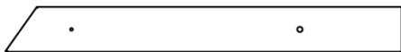
H4 | SUPPORT DE TOIT - W104024 (x2) | 1 po x 3 3/8 po x 29 5/8 po (24 x 86 x 752)
