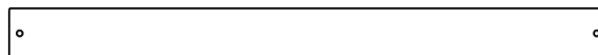
H11 | SUPPORT DE PLANCHER - W4L16355 (x1) | 1 po x 3 3/8 po x 40 3/8 po (24 x 86 x 1024)
