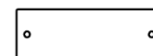
M3 | LISSE MURALE COURTE - W4L16354 (x2) | 5/8 po x 3 3/8 po x 10 po (16 x 86 x 254)
