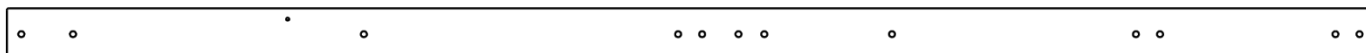
E6 | MONTANT DU FORT - W4L16347 (x1) | 1 3/8 po x 3 3/8 po x 89 1/2 po (36 x 86 x 2274)
