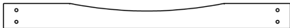
M10 | LISSE MURALE DE ARCHE - W103987 (x1) | 5/8 po x 3 3/8 po x 37 1/2 po (16 x 86 x 952)
