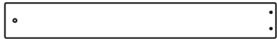
M8 | LAMELLE MURALE - W104001 (x4) | 5/8 po x 3 3/8 po x 25 5/8 po (16 x 86 x 650)
