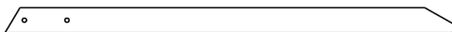
F3 | CALE ANGULAIRE STANDARD - W4L16343 (x1) | 1 3/8 po x 2 3/8 po x 41 3/8 po (36 x 60 x 1052)
