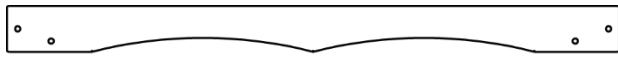
H13 | PLANCHE D'ARCHE DOUBLE - W103990 (x1) 1 po x 3 3/8 po x 45 3/8 po (24 x 86 x 1154)
