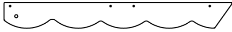
H3 | SUPPORT DE TOIT - W104017 (x2) | 1 po x 3 3/8 po x 29 5/8 po (24 x 86 x 752)
