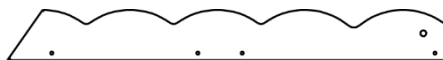
H3 | SUPPORT DE TOIT - W104017 (x6) | 1 po x 3 3/8 po x 29 5/8 po (24 x 86 x 752)
