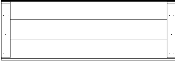
RP2 | PANEL DE TECHO - W104016 (x1) | 1 5/8"x15 5/8"x46" (42x396x1168)
