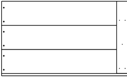
RP5 | PANEL DE TECHO - W104022 (x1) | 1 5/8"x15 5/8"x46" (42x396x672)
