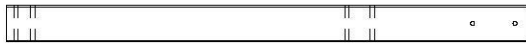
SP50 | SOPORTE DE LA VIGA DEL COLUMPIO - W4L16085 (x1) 3 3/8"x3 3/8"x49 3/8" (86x86x1254)
