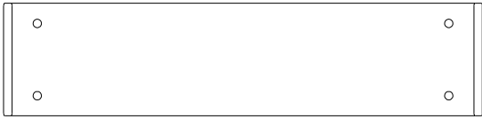
G2 | GROUND BOARD - W4L04459 (x1) | 1"x5 1/4"x22 3/8" (24x134x570)
