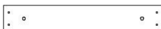
H77 | PLANCHE DE FIXATION - W4L15929 (x1) | 1 po x 3 3/8 po x 20 1/8 po (24 x 86 x 512)
