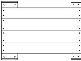
WP8 | PANNEAU MURAL - W2A01409 (x1) | 1 5/8 po x 19 po x 26 1/8 po (40 x 482 x 664)
