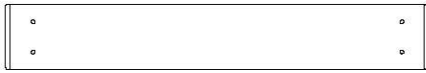
M5 RAIL MURAL - W4L04465 (x1) 5/8 po x 3 3/8 po x 22 po (16 x 86 x 563)
