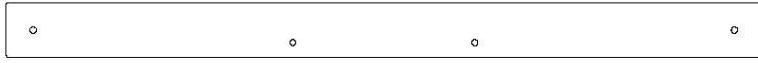
H5 | RAIL DE PLATEFORME - W4L16094 (x1) | 1 po x 3 3/8 po x 47 3/8 po (24 x 86 x 1204)
