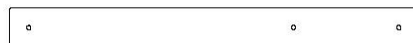
M3 | RAIL MURAL - W4L16096 (x2) | 5/8 po x 3 3/8 po x 35 1/4 po (16 x 86 x 896)
