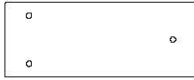
K7 RAIL MURAL - W4L04488 (x2) 5/8 po x 5 1/4 po x 13 1/2 po (16 x 134 x 344)
