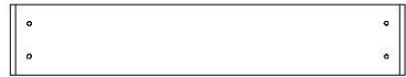
M8 RAIL MURAL - W4L04466 (x1) 5/8 po x 3 3/8 po x 18 3/4 po (16 x 86 x 475)
