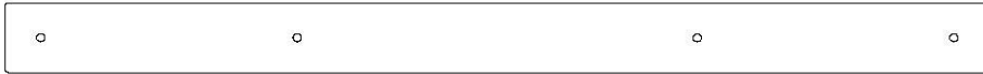
H3 RAIL DE PLATEFORME - W4L04462 (x1) 1 po x 3 3/8 po x 47 3/8 po (24 x 86 x 1204)
