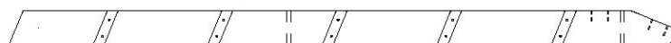
E78 | MONTANT DROIT - W4L15933 (x1) | 1 3/8 po x 3 3/8 po x 64 3/8 po (36 x 86 x 1634)
